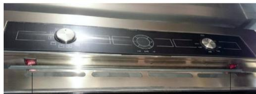
This switch is controlling the warming element in the bottom oven element (200 watt)
