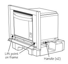
Remove all packing material. Review installation instructions. Lower drip tray door and lift from these points for installation.
