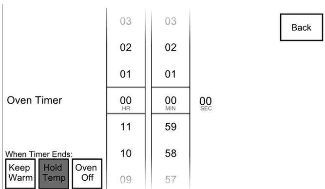
Keep Warm™ setting will reduce the oven temperature to 170°F (77°C) after the cook time ends. Hold Temp will keep the set oven temperature after the cook time ends. Oven Off will turn the oven off when the cook time ends.
