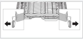
Remove the top cutlery tray. Push the top spray arm up and turn the spray arm bearings counterclockwise to remove the spray arm.
