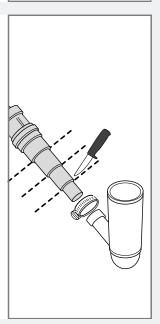
The drain hose can also be connected to a connection nipple on the sink unit's water trap. The connection nipple must have an internal diameter of at least 1/2".
