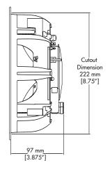
The DI 8R *Disappearing* TM *In-Wall* speaker features near-invisibility thanks to its small diameter, hidden flange design, and low-profile micro-perf grille. It is as easy to install as traditional flanged flush-mount speakers, and doesn't require custom sheetrock/spackle skills to install, yet it looks practically invisible when installed in a ceiling.
