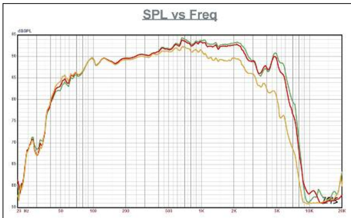
Frequency response of driver with conventional phase plug: @ 0° (green), -15° (red) and -30° (yellow). Notice the severe high-frequency roll-off at 30 degrees off axis.
