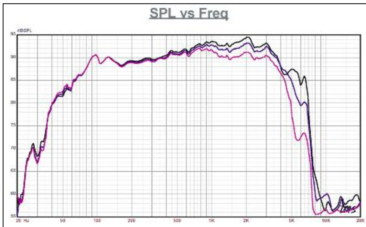
Frequency response of a BDSS driver with LRW phase plug: @ 0° (black), -15° (blue) and -30° (red). Even at 30 degrees off axis, the response is, at most, only 3dB down from the on-axis response.
