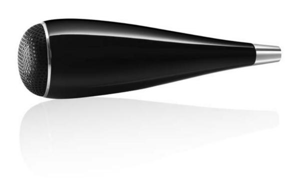
**Solid body tweeter** Vibration is the enemy of good sound. To minimise vibrations, you need components that are as stiff as possible. For the 800 Series Diamond, we created our stiffest tweeter enclosure yet. The tweeter assembly for the new range is housed in a solid piece of aluminium, while an improved gel decoupling system isolates the tweeter from the effects of cabinet resonance. The result? Pin-sharp acoustic detail, and new levels of insight into a musical performance.
