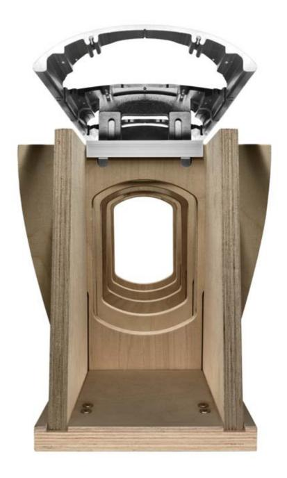
Matrix™ Matrix provides the backbone for our speakers. It's an internal structure that works like the bracing of a ship's hull, with criss-crossed interlocking panels keeping our cabinets rigid and inert. For the 800 Series Diamond, we've introduced our most radical rethink of the Matrix concept yet. The internal panels are thicker, solid plywood has replaced MDF, and metal components have been added to reinforce key stress points. All together it's the most solid Matrix system we've ever built.
