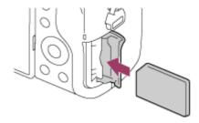
With the notched corner facing in the direction illustrated, insert the memory card until it clicks into place. Insert the memory card correctly. Not doing so may cause a malfunction.
