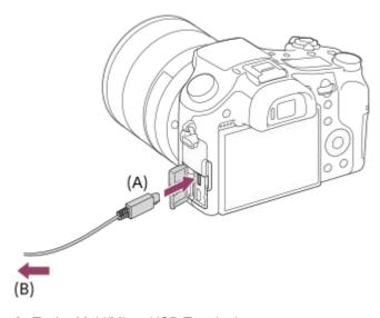
**A:** To the Multi/Micro USB Terminal **B:** To the USB jack of the computer
