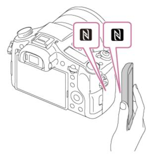
The product and the smartphone are connected, and PlayMemories Mobile automatically launches on the smartphone, and then the displayed image is sent to the smartphone.
