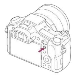
The exposure is locked, and  $\bigstar$  (AE lock) is displayed.
