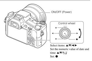
1 Set the ON/OFF (Power) switch to ON.
