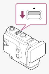
• When using FDR-X3000/HDR-AS300 with the Underwater Housing supplied with HDR-AS50, detach the adaptor (A) from the Underwater Housing.
