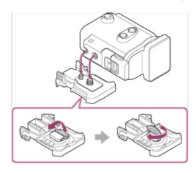
2 Attach the attachment buckle to the accessory by sliding it until it clicks into place.
