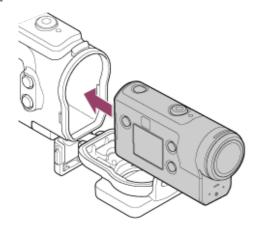
Insert the tab of the case body into the slot of the case cover.
