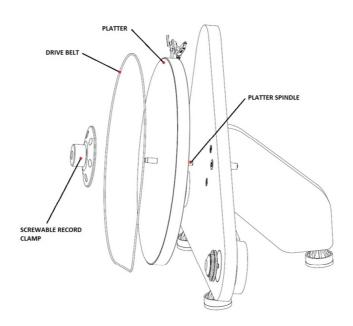
After placing the record on the platter, it is necessary to tighten the screw-able record clamp (6) onto the platter spindle.
