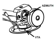
With the aid of a good magnifying glass adjust the needle until it is vertical in the groove (i.e. perpendicular to the record's surface). Ideally this should correspond to the top surface of the cartridge body being parallel to the record surface, but in practice this is often not the case.
