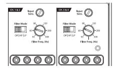
To properly set the amplifier for maximum clean output, please refer to Appendix A (page 14) in this manual. After using this procedure, you can then adjust the "Input Sens." levels downward if this is required to achieve the desired system balance.
