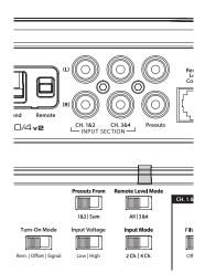
If you wish to send four discrete channels into the XD400/4, simply use all four inputs and set the "**Input Mode**" switch in the "**4** Ch." position.
