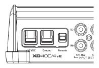
The XD400/4v2's "+12 VDC" and "Ground" connections are designed to accept 4 AWG power wire. 8 AWG is the minimum required wire size for this amplifier.
