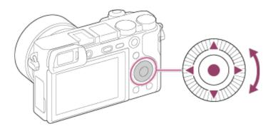
You can select setting items by turning or pressing the top/bottom/right/left side of the control wheel. Your selection is determined when you press
