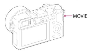
To adjust the shutter speed and aperture value to the desired settings, set the shooting mode to 🖽 (Movie).
