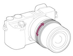
• When you rotate the focus ring, the focus distance is displayed on the screen.
