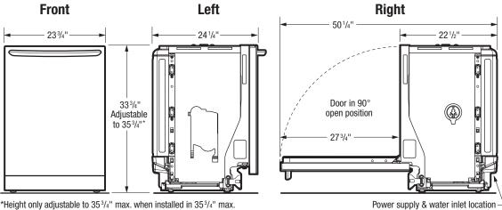
standard cabinetry cutout. (Dimensions do NOT include insulation insulation blanket may be compressed during installation.)
