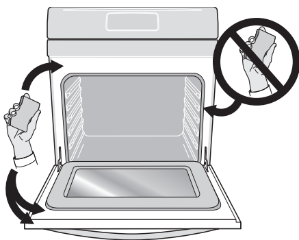
Figure 16: Clean around the oven door gasket
