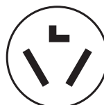
3-wire receptacle (10-30R)
