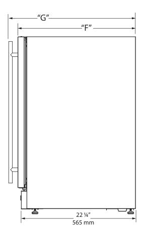
Minimum rough-in opening is required to be larger than the adjusted height of the cabinet.
