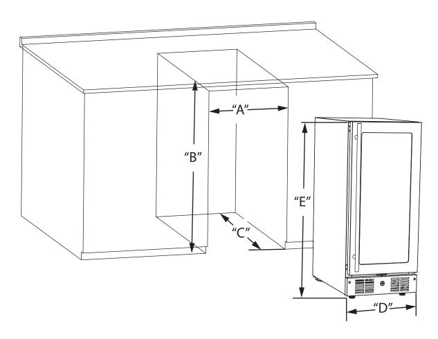
If necessary, to gain clearance inside the rough-in opening, a hole can be cut through the adjacent cabinet and the power cord routed through this hole to a power outlet. Another way to increase the available opening depth is to recess the power outlet into the rear wall to gain the thickness of the power cord plug. Not all recessed outlet boxes will work for this application as they are too narrow, but a recessed outlet box equivalent to Arlington #DVFR1W us recommended for this application.
