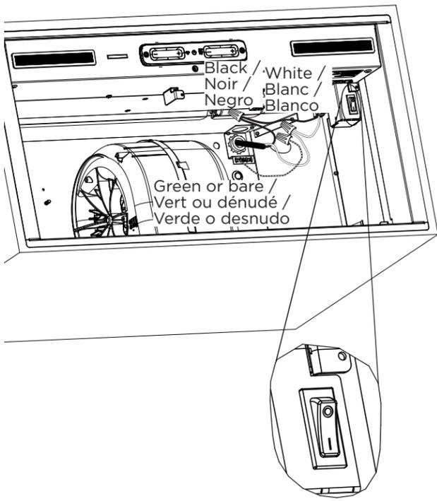
NOTE: Make sure the main power switch is set to position 1.
