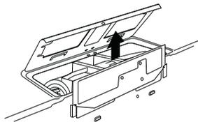
3. Carefully pull out the blower unit. The wires will extend far enough to allow you to adjust the blower unit.
