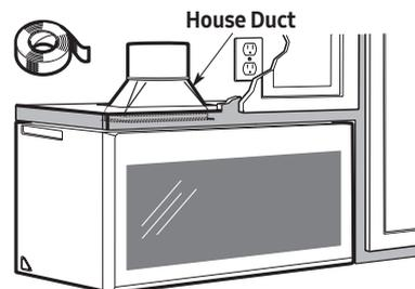
1. Extend the house duct down to connect to the exhaust adaptor.
