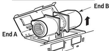
**CAUTION:** To avoid breaking or cracking the blower blade, do not touch the blade. Hold the outer case of the blower when you pull it out or put it back in place.
