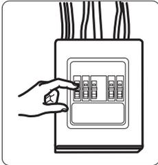
**CAUTION:** For personal safety, remove house fuse or open circuit breaker before beginning installation to avoid severe or fatal shock injury.
