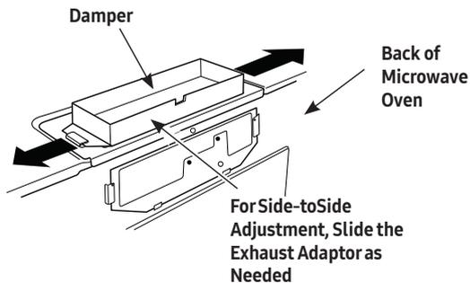
**NOTE:** You must attach the house duct to the exhaust adaptor after installation is complete.
