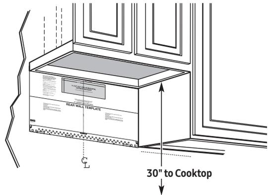
Draw a vertical line on the wall at the center of the 30" wide space. Tape the Rear Wall Template onto the wall so that the top of the template touches the bottom of the cabinet frame and the centerline on the template lines up with the line you drew on the wall.
