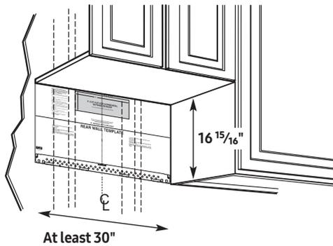
Draw a vertical line on the wall at the center of the 30" wide space. Tape the Rear Wall Template onto the wall so that the top of the template touches the bottom of the cabinet and the centerline on the template lines up with the line you drew on the wall.
