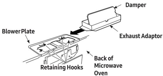
1. Slide the exhaust adaptor as shown in the diagram above.
