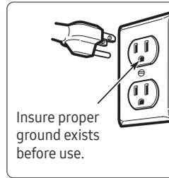
**The power cord of this appliance is equipped with a three-prong (grounding) plug which mates with a standard three-prong (grounding) wall receptacle to minimize the possibility of electric shock hazard from this appliance.**
