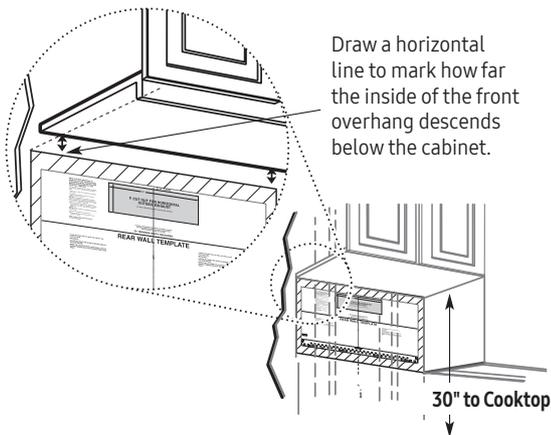
Draw a horizontal line to mark how far the inside of the front overhang descends below the cabinet.
