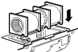
**CAUTION:** Do not pull or stretch the blower unit wiring. Make sure the wires are not pinched.
