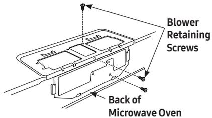
2. Open the blower door by lifting it up at the back of the microwave. Remove and save the blower shield on the back of the microwave by sliding it up. Remove and save the metal vent fan cover on the back of the microwave by sliding it up.
