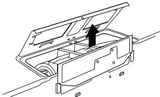
7. Close the blower door. Slide blower shield onto the top of the blower door opening.
