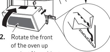
2. Rotate the front of the oven up against the cabinet bottom.
