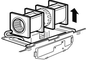
**CAUTION:** To avoid breaking or cracking the blower blade, do not touch the blade. Hold the outer case of the blower when you pull it out or put it back in place.
