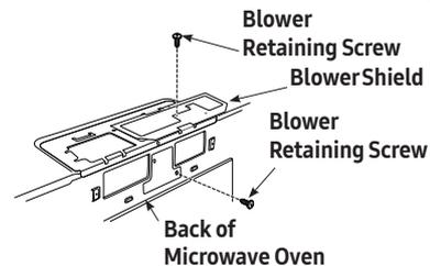
8. Slide the exhaust adaptor onto the back of the microwave oven, securing it into the lower locking tabs. Take care to ensure that the damper hinge is installed so that it is at the top and that the damper swings freely. Reinstall the upper blower motor screw through the adaptor and the blower door and into the back of the microwave oven.
