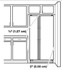
To ensure proper ventilation for your refrigerator, allow for ½" (1.27 cm) of space on each side and at the top. Allow for 1" (2.54 cm) of space behind the refrigerator. If your refrigerator has an ice maker, allow extra space at the back for the water line connections. When installing your refrigerator next to a fixed wall, leave a 2" (5.08 cm) minimum space on each side (depending on your model) to allow the doors to swing open.
