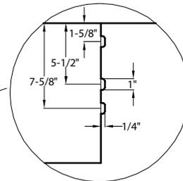
NOTE: IF EXISTING ISLAND CUTOUT IS EXACTLY THE MINIMUM DIMENSION SHOWN (FOR WIDTH), THEN A SMALL RELIEF NEEDS TO BE CUT IN THE FRONT VERTICAL EDGES OF THE ISLAND (BOTH SIDES) APPROX. 1" BACK FROM THE FRONT.
