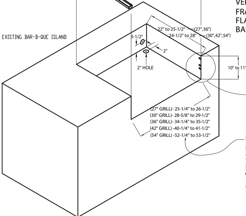
1) AFTER COMPLETE ASSEMBLY (PAGE 1) PLACE LYNX ISLAND ADAPTOR FRAME DIRECTLY OVER ISLAND CUTOUT. PLACE FRONT EDGES OF SIDE EXTENSIONS FLUSH WITH FRONT OF ISLAND FACE. CENTER FRAME LEFT TO RIGHT OVER ISLAND CUTOUT.
