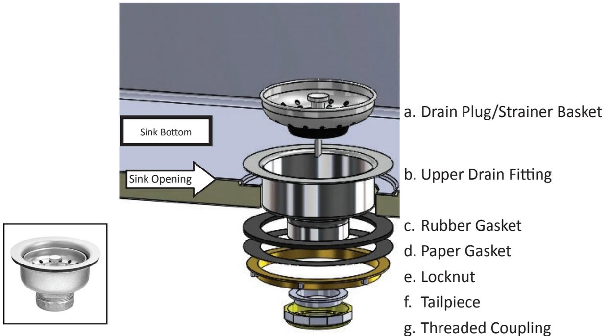
2. Remove the drain plug strainer basket (a) and separate the upper drain fitting (b) from the remainder of the drain assembly.
