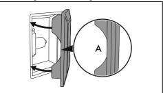
7. Press the cover firmly so that it adheres tightly to the light bulb holder.
