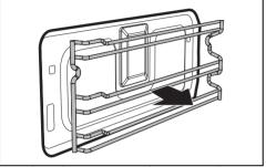
When cleaning is complete, repeat the above procedures to put the guide frames back in.
