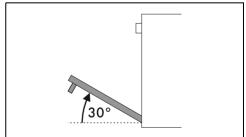
To reattach the door, insert the hinges into the slots on the oven, making sure that grooved sections A fit tightly in the slots.
