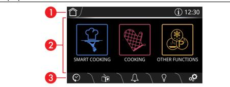
The parameters and values for the currently selected function will be indicated on the display. To use it, simply touch the "virtual" buttons and/or scroll through the values shown (the picture shows the main menu screen).
