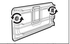
2. Pull the frame towards the inside of the oven to free it from the fastening pins.
