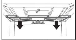
When you have finished cleaning, place the heating element back in position and turn the retaining latch to lock it in place.
