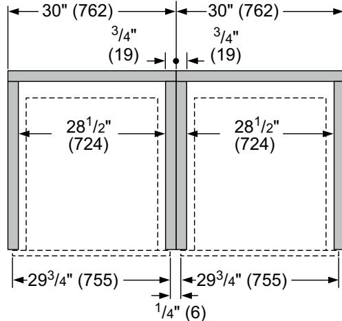
**Flush side-by-side installation**
