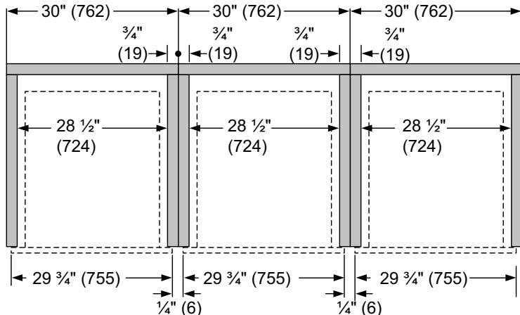
Flush side-by-side-by-side installation
