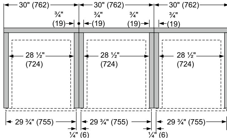
Instalación enrasada side-by-side-by-side
