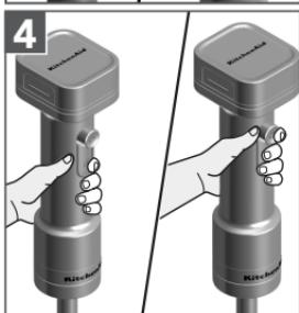
4 Insert the Cordless Hand Blender into the mixture. Press and hold the Unlock Button first, then the Variable Speed Controller to start.
