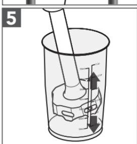
5 Use the draw up motion with the Cordless Hand Blender to move the ingredients within the Jar. Slowly draw it upwards against the side of the Jar. Repeat the process until the ingredients are at the desired consistency.
