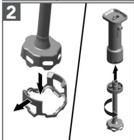
2 To insert the Pan Guard, angle the Blending Arm to one side of the mounting clip. Then, gently pull the other mounting clip outward and push down the Blending Arm. Insert the Blending Arm into the handle and twist to lock.
