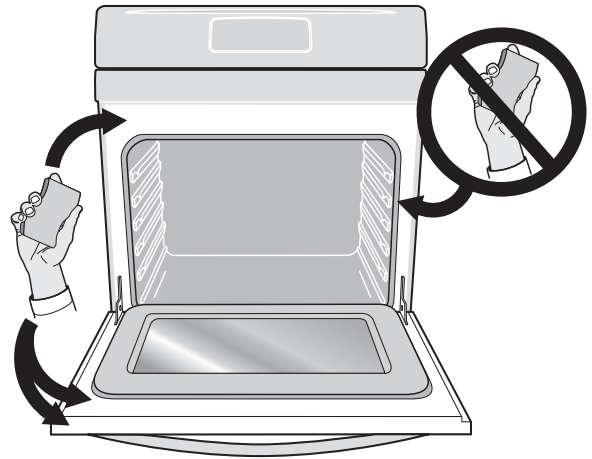
Figure 6: Clean around the oven door gasket
