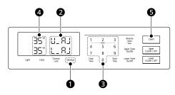
To adjust the lower oven, press the Settings button ① repeatedly until L\_RJ ②shows in the display. To adjust the upper oven, press the Settings button ① repeatedly until U\_R J ③shows in
