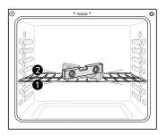
**2** If the level doesn't show that the rack is level, adjust the leveling legs with a wrench.
