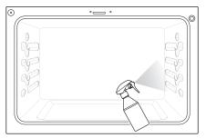
5 Spray or pour the remaining water (8 oz or 240 ml) onto the bottom center of the oven cavity. The indentation on the oven bottom should be fully covered to submerge all soils. Add water if necessary.
