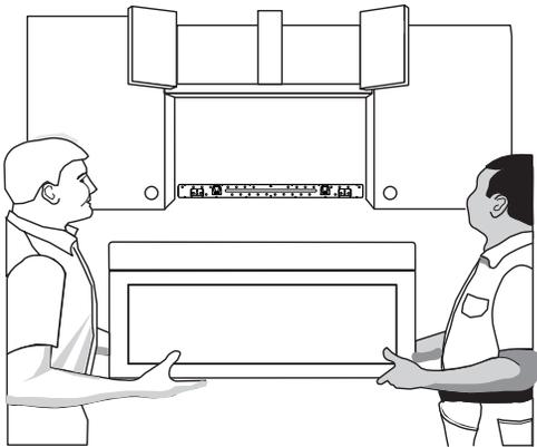
3. Using 2 or more people, lift microwave oven and hang it on support tabs at the bottom of mounting plate.
