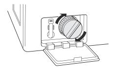
**8** Close the drain pump filter cover.
