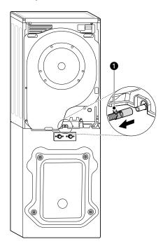
Connect the drain hose of the dryer and secure the hose clamp.
