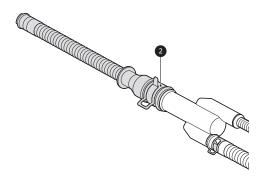
Securely connect the short drain hose to a floor drain or standpipe. When connecting to a waste spigot, use a band clamp 3 on the end of the short drain hose.
