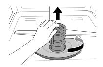
Clean the filters with a soft brush under running water. Reassemble the filters before reinstalling them.
