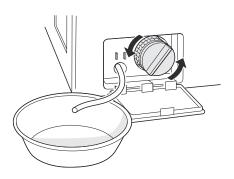
**5** Clean the pump filter and opening.
