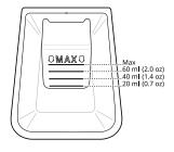
If you use a detergent that does not dissolve easily or a detergent with high viscosity, it will leave a residue and clog the dispenser.
