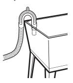
Use the provided tie strap to secure the drain hose in place.
