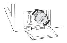
Close the drain pump filter cover.
