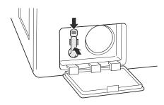
7 Insert the drain pump filter and twist it clockwise.
