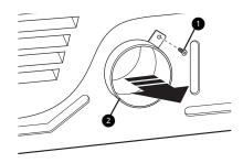
Press the tabs on the knockout and carefully remove the knockout for the desired vent opening. (Right-side venting is not available on gas models.) Press the adapter duct onto the blower housing and secure to the base of the dryer as shown.
