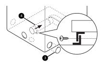
Preassemble a 4" (10.2 cm) elbow **5** to the next 4" (10.2 cm) duct section, and secure all joints with duct tape. Be sure that the male end of the elbow faces AWAY from the dryer. Insert the elbow/duct assembly through the side opening and press it onto the adapter duct. Secure it in place with duct tape. Be sure that the male end of the duct protrudes 1.5" (3.8 cm) to connect the remaining ductwork. Attach the cover plate **6** to the back of the dryer with the included screw.
