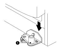
2 Fit the hinge 2 over the hinge lever latch 3 and slot it into place. Rotate the lever 4 counterclockwise to secure the hinge.
