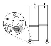
Open the door and use the wrench to loosen the keeper nut by turning it to the left.
