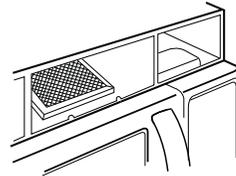
7. Slide the bottom of the vent cover into place. Push the top until it snaps into place. Replace the mounting screws. Turn the power back on at the main power supply and set the clock.
