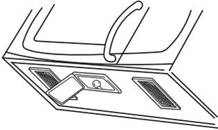
3. Replace bulb with 30 watt appliance bulb.
