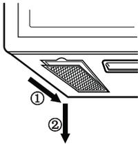
2. Soak grease filters in hot water and a mild detergent. Rinse well and shake to dry. **Do not use ammonia or place in a dishwasher. The aluminum will darken.**
