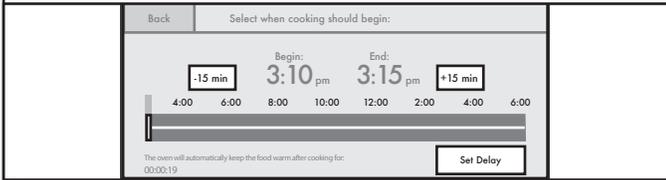
Touch the 15 Min keypad(s) or slide the bar. The difference between the start and end times should equal the cook time.
