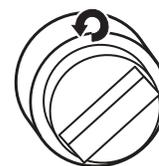
If the burner does not light, check cap alignment. If the burner still does not light, do not service the sealed burner yourself. Contact a trained repair specialist.
