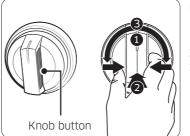
Make sure all surface burners are properly installed. To light a burner:
