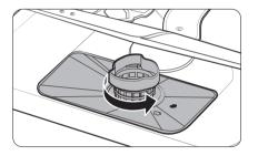
rack. The lower nozzle is visible on the bottom.2. Unclog and clean the nozzle.
