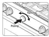
The dial knob can be manipulated as following methods: turning and pushing.
