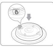
**2.** Install the burner head so that the electrode passes through the opening for the electrode. Make sure the burner head lies flat on the stove top.
