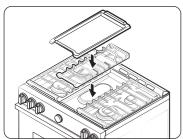
The griddle can be used only with the center burner on the center grate. Use caution when putting the griddle on the center grate.
