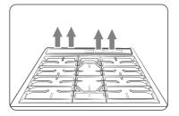
The Oven/Cooling vents are located at the back of the oven range. Proper air circulation prevents combustion problems and ensures good performance.
