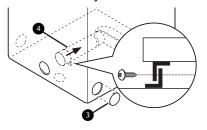
3 Preassemble a 4" (10.2 cm) elbow to the next 4" (10.2 cm) duct section, and secure all joints with duct tape. Be sure that the male end of the elbow faces AWAY from the dryer. Insert the elbow/duct assembly through the side opening and press it onto the adapter duct. Secure it in place with duct tape. Be sure that the male end of the duct protrudes 1.5" (3.8 cm) to connect the remaining ductwork. Attach the cover plate to the back of the dryer with the included screw.
