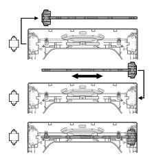
• Now rotate the **①** hinge filler 180 degrees and install it on the upper left side of the door.
