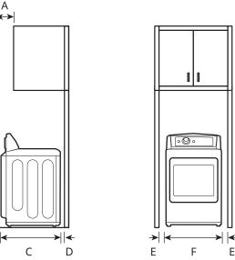
For cabinet installation with a door, minimum ventilation openings in the top of the cabinet are required.
