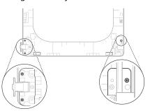
2) Rotate the **O** lower hinge assembly 180 degrees and install it on the right side using the two screws removed in a previous step.
