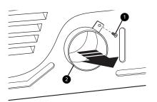
2 Press the adapter duct ③ onto the blower housing and secure it to the base of the dryer as shown.
