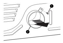
2 Press the tabs on the knockout **3** and carefully remove the knockout for the desired vent opening. (Right-side venting is not available on gas models.) Press the adapter
