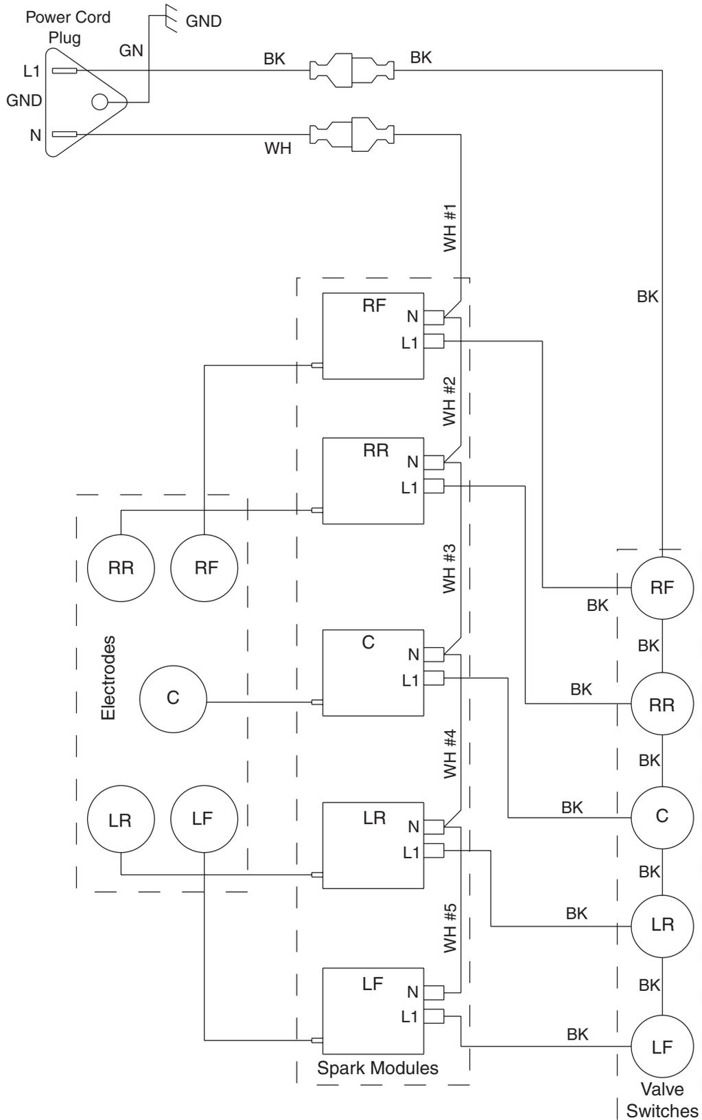
**NOTE:** Electric circuit is closed when knob is pushed in and rotated from 0° to 210° counterclockwise from OFF.
