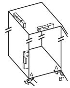
▶ Then prop up the door: Screw out the adjustable foot on the bearing bracket (B) using the open-ended wrench SW10 until it comes into contact with the floor, then turn an additional 90°.
