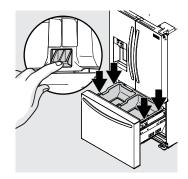
4. Lift the basket up and out of the freezer compartment.
