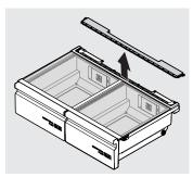
Removing Auto Humidity Control Membrane
