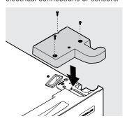
After you remove the hinge covers, disconnect any harnesses between the cabinet and doors by grasping both sides of the connector firmly, depressing the latch and pulling it apart.
