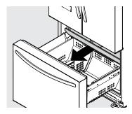
Slightly push inward on the basket tabs to release the upper basket from the slide assemblies (one per side, in front).
