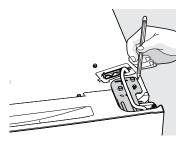
4. Remove the bulkhead cover at the rear of the unit to access the water tube. Disconnect the water tube at the push-lock connection on the rear of the unit below the bulkhead. The dispenser line is connected to the yellow water line coming from the main water valve.
