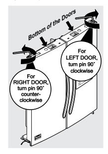
Once you reset the door pins, follow the steps **To reinstall the refrigerator doors**.
