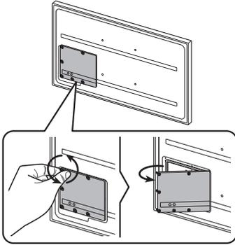
2. Remove the appropriate silicone bar for the thickness of the cable to connect.
