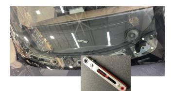
5 Secure all Alpine speakers to the dash by Re-installing all remaining factory T20 Torx. After speakers are mounted Install the dashboard speaker cover panel by applying uniform pressure to engage the factory clips.
