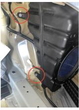
5 Re-install the factory amplifier and bolts if premium equipped.
