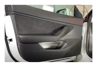
**3** Unclip the Factory Tweeter from the Housing by gently twisting and pulling.
