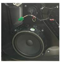
5 Plug in all remaining factory door connectors. Mount and re-install each factory door panel using (3) T30 Torx. Apply Pressure around the door panel to engage the factory clips. Re-install the Red Reflector Clips 2 Use a Panel Removal Tool around the edge of the panel to release the factory clips. Release the panel and pull upwards to detatch, un-plug the factory panel connections including the green speaker plug
