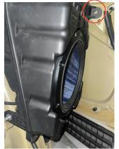
6 Re-connect the factory subwoofer plug, place the carpet into position and re-install the upper and lower plastic trim panels.
