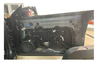
4 Install the new Alpine Speaker & Adapter to the door panel using the factory screws. Plug in green speaker adapter plug
