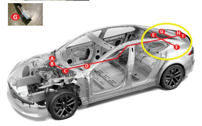
7 Route cable G behind the trunk lining trim, (Plug G) connects to the subwoofer enclosure located behind the rear passenger tire well.
