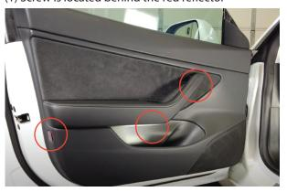
**3** Remove 4 bolts securing each factory speaker adapter. Use 8mm Socket or T25 Torx (Varies depending on year) The factory Adapter should then unclip easily.
