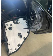
4 Using hand screw driver nstall the new Alpine Speaker to the door panel using the (6) supplied phillips tapping screws & Plug in the speaker connector
