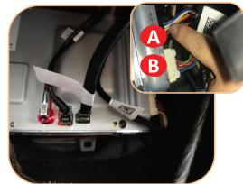
4 Remove the passenger side baseboard lower door trim and locate the connector just before the base of the B-pillar. Transfer the connections to (Plug D)
