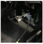
3 Connect Harness "K" black plastic molex end with corresponding plug of CANPRO CP1-S Module "L". Set dipswitch 2 to ON position
