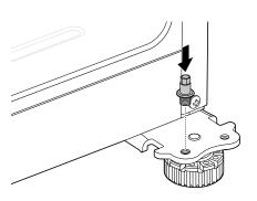
6 Using a 3/8 in. socket wrench with a 2-inch extension, loosen the 2 bolts on the bottom hinge bracket. Use a Phillips screwdriver to loosen the screw.
