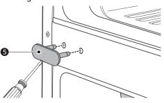
8 Remove the decorative screw <sup>(3)</sup> located on the housing between the freezer and refrigerator doors. (You will need this hole for the middle hinge bracket.)
