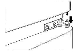
**3** Carefully snap the top hinge cover back into place over the hinge.
