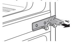
Using a 1/4 in. socket wrench, loosen and remove the bottom hinge pin 4 from the bottom hinge bracket 5. Remove the washer from the bottom hinge pin and set it aside.
