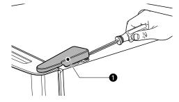
2 Use 10 mm or 3/8 inch socket wrench, remove the three bolts and lift off the top hinge ②. Set parts aside.
