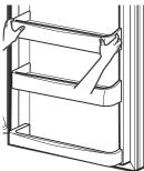
2 To assemble the bin, slide it in above the desired support and push down until it snaps into place.
