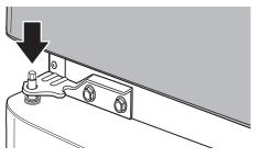
**3** Place the top hinge on top of the freezer door and line up the top hinge with the holes on top of the refrigerator. Use the three bolts to attach the hinge.
