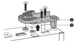
6 Move the bracket to the opposite side of the door and insert the hinge pin sleeve. Reverse the hinge lever ④ by flipping it over. Place it on top of the bracket, and tighten both down with the screw. Then insert the remaining 2 screws to tighten the bracket to the refrigerator door.
