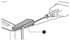
Using 10 mm or 3/8 inch socket wrench, remove the three bolts and lift the top hinge
