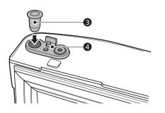
7 Reverse the hinge lever **S** by flipping it over. Place it on top of the bracket and tighten both down with the screw.
