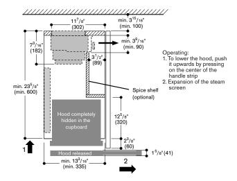
Cross-section of upper cabinet with AA 211 812 air recirculation module
