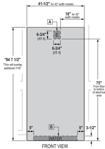
A – Mounting the junction in this location will also allow for front accessibility through access panel.
