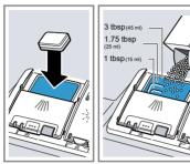
If you are using tablets, one is enough. Insert the tablets in a horizontal position.
