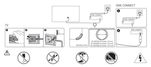
Refer to the figures and connect the One Clear Connection, supplied as an accessory, to the TV and the One Connect.
